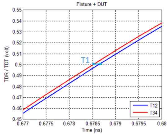
Figure 19. Computing total skew (T1) of fixture + DUT from TDT.
