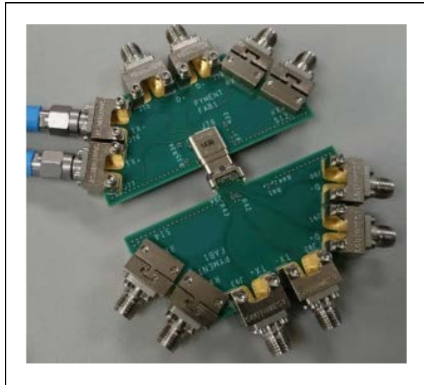
Figure 6: USB Type-C connector (DUT) and fixture.
